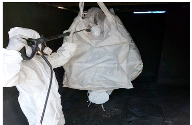
Pic 4. Empty bags are washed then sold to non-food packaging applications. The washing water is tested for any residual material before the bags are declared fit for sale.
