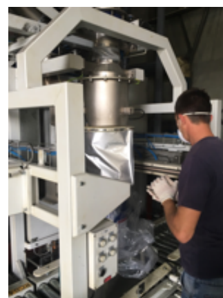
Fig 6b: Automated drum filling station: Finished product is filled into drums with efficient dust collection and without operator exposure.
