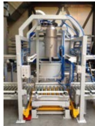
Fig 6: Drum filling station: Finished product is filled into drums with efficient dust collection and without operator exposure.
