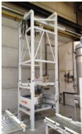
Fig 5: Big bag discharge station: Raw material is fed from big bags into the reduction furnace without operator exposure.
